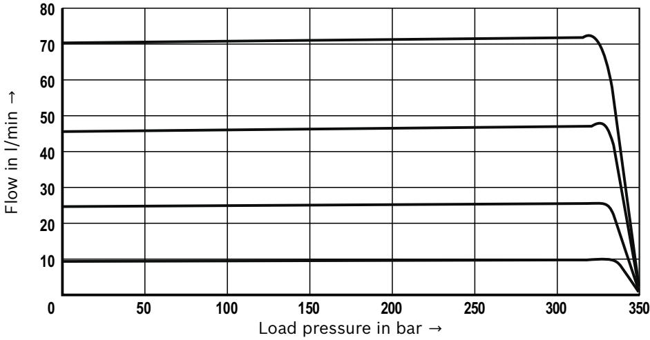
Regulated flow at main port ③ as a function of the load pressure 3-way function (main port ② open to the tank)
