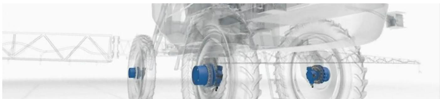
Especially in agricultural sprayers, the advantages of the internal multi-disc brake come fully to bear. It is lighter in weight than conventional designs and its protection against grime greatly reduces the need for maintenance.
