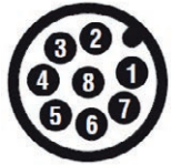
(Connector) M12x1; 8-pole, A-coded
