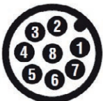
(Connector) M12x1; 8-pole, A-coded
